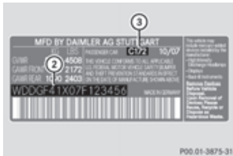
Example: vehicle identification plate (USA only)
